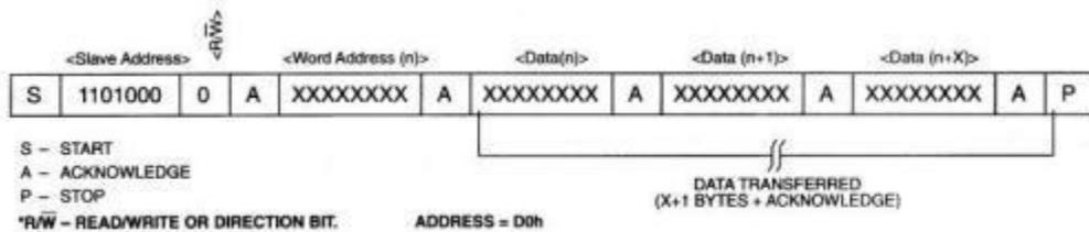
2. **Slave transmitter mode( 1307 read mode) :** The first byte is received and handled as in the slave receiver mode. However, in this mode, the \*direction bit will indicate that the transfer direction is reversed. Serial data is transmitted on SDA by the 1307 while the serial clock is input on SCL.
