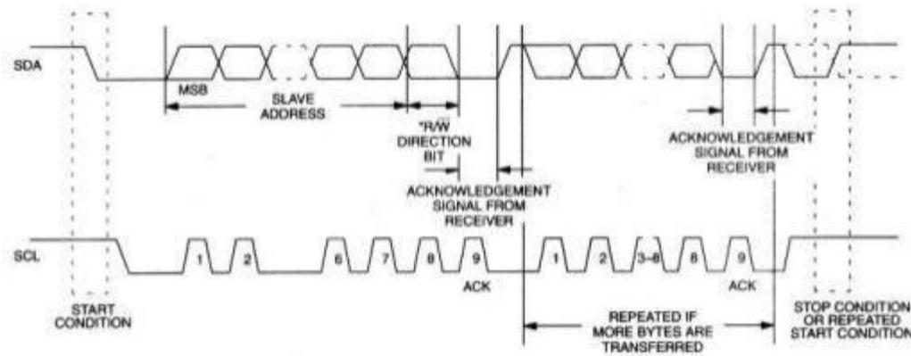
Depending upon the state of the R/W bit, two types of data transfer are possible:
