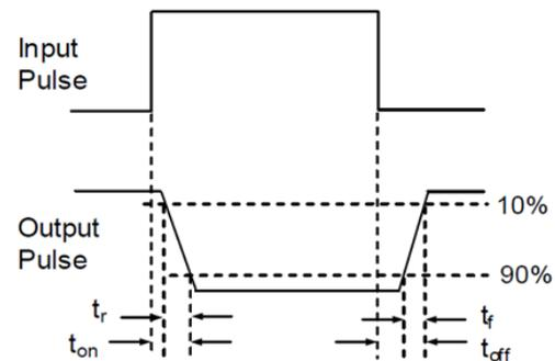
Figure 10. Switching Time Test Circuit & Waveforms
