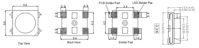
Remarks: Dimension of 5.0\*5.4\*1.57mm, default Tolerance of 0.05mm.
