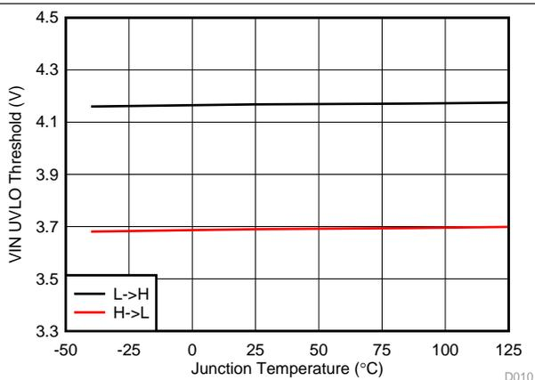
Figure 10. VIN UVLO Threshold vs Junction Temperature
