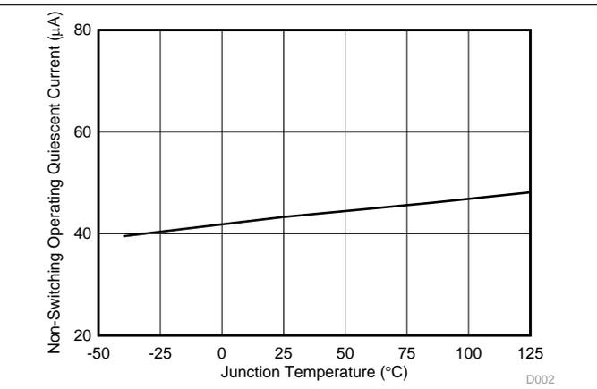
Figure 2. Non-Switching Operating Quiescent Current vs Junction Temperature
