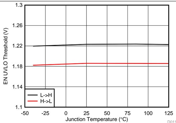
Figure 11. EN Threshold vs Junction Temperature
