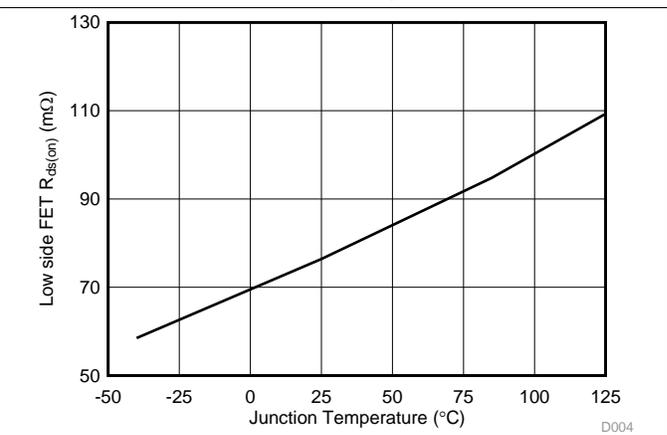
Figure 4. Low-Side FET On Resistance vs Junction Temperature
