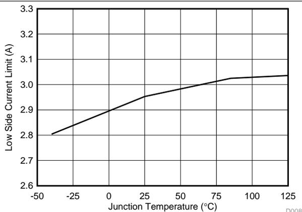
Figure 8. Low-Side Current Limit Threshold vs Junction Temperature
