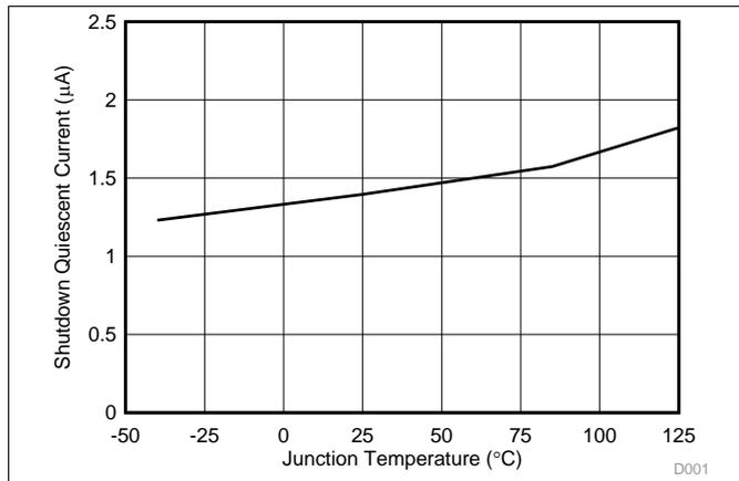
Figure 1. Shutdown Quiescent Current vs Junction Temperature
