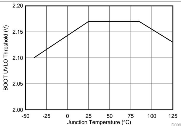
Figure 9. BOOT-SW UVLO Threshold vs Junction Temperature
