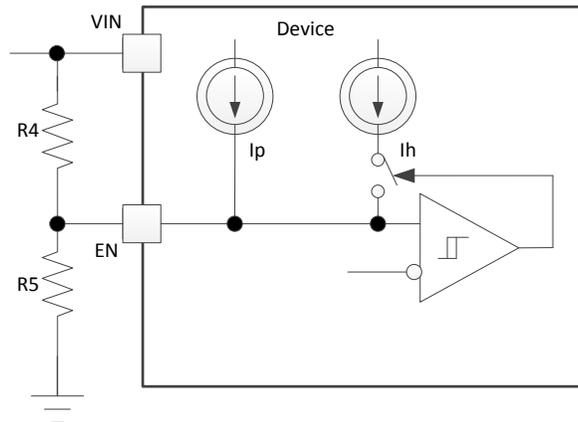
**Figure 13. Adjustable VIN Undervoltage Lockout**
