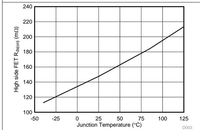
Figure 3. High-Side Resistance vs Junction Temperature
