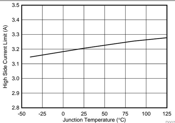
Figure 7. High-Side Current Limit Threshold vs Junction Temperature
