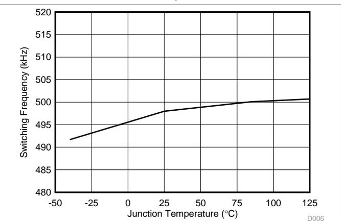
Figure 6. Centre Switching Frequency vs Junction Temperature
