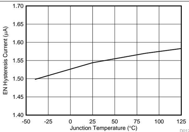
Figure 12. EN Hysteresis Current vs Junction Temperature
